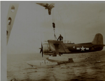
LTJG Earles attaches cables and lines to prepare for hoisting.
